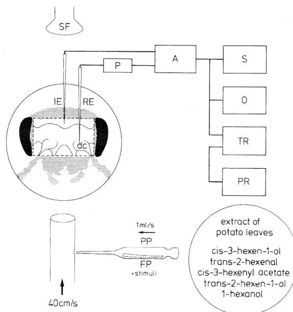
Fig. 2. Schematic representation of the experimental set-up. A, amplifier; dc, deutocerebrum; FP, filter paper; IE, indifferent electrode; O, oscilloscope; P, probe; PP, Pasteur pipette; PR, paper recorder; RE, recording electrode; S, speaker; SF, suction funnel; TR, tape recorder.
