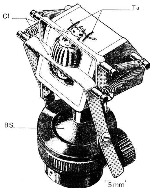
Fig. 1. Stainless-steel holder for mounting the beetles during intracellular recordings of deutocerebral neurones. BS, ball-and-socket joint; Cl, clamps; Ta, tape.
