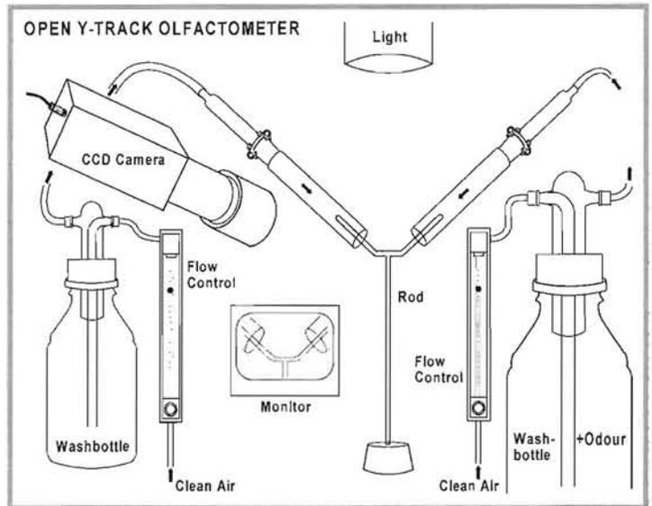
Figure 4 - An olfactometer to measure the behavioural response of aphids to plant odours. An aphid released at the base of the rod, will walk upwards and at the junction, has to decide to walk towards the odour or the control side.
